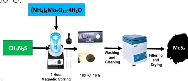
Figure 1: Schematic diagram of the synthesis of MoS 2 nanosheets
